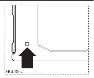
2 When charging the LED light above the micro-USB jack (Figure C) will be solid RED and GREEN indicating charged.
