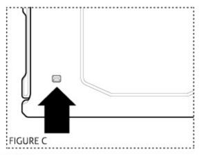
2 When charging the LED light above the micro-USB jack (Figure C) will be solid RED and GREEN indicating charged.
