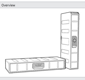
**Vertical Orientation!** The safe must be securely mounted on the wall to prevent the safe from falling.
